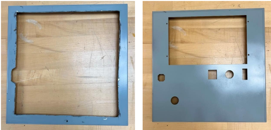
Cabinet door with cut out (left); cabinet door with HMI door panel mounted (right).
